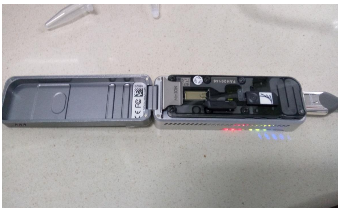
Figure 1: MinION sequencing device
